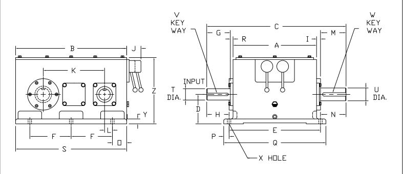
Center Distance Between Shafts, Shaft Diameters, and Distance from Center Line of Shaft to Base May Vary Depending on Application.
