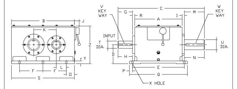
Center Distance Between Shafts, Shaft Diameters, and Distance from Center Line of Shaft to Base May Vary Depending on Application.
