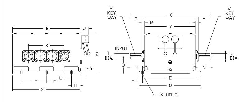
Center Distance Between Shafts, Shaft Diameters, and Distance from Center Line of Shaft to Base May Vary Depending on Application.
